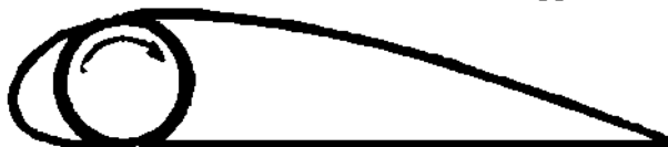
Figure 1: Airfoil with the rotating cylinder at the nose, proposed by Prandtl [1]
