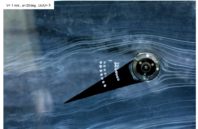
Figure 11: Cylinder rotating at \bar{U} = 5 , \alpha = 25^\circ
